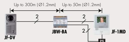
PS : Power supply PS-1820S, PS-1820UL, PS-1820, PS-1810DIN PT : AC transformer
