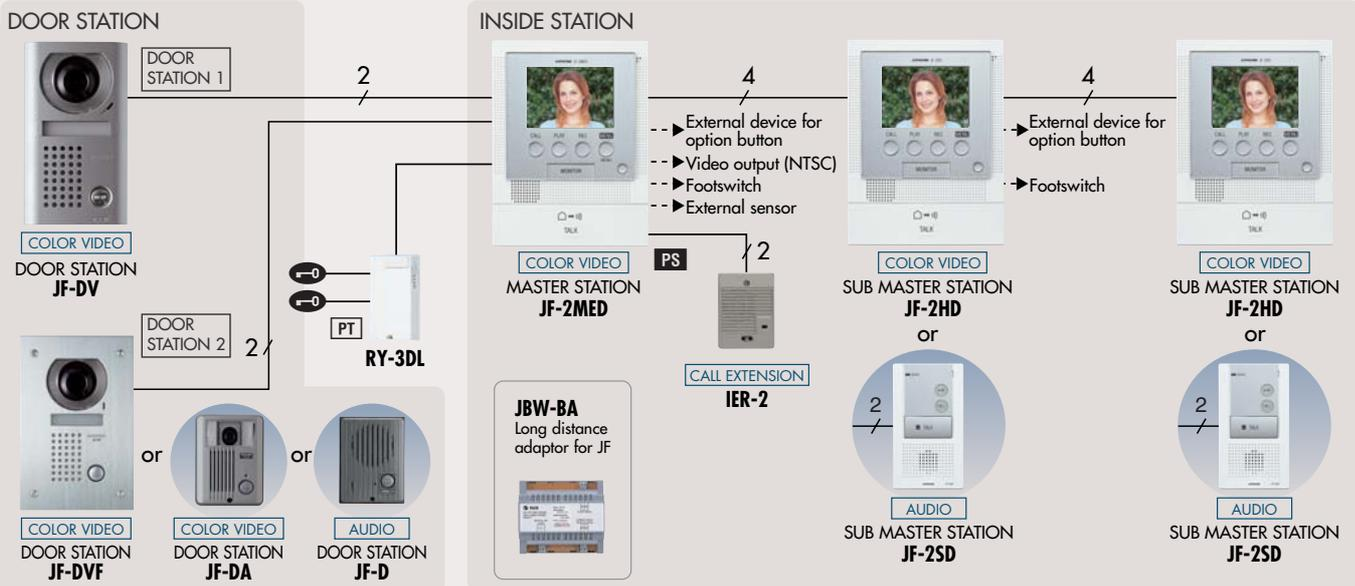
PS : Power supply PS-1820S, PS-1820UL, PS-1820, PS-1810DIN PT : AC transformer
